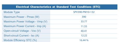
Tolerance of Rating Pmax /Voc/ lsc[%]: ±5/ ±4/ ±4
